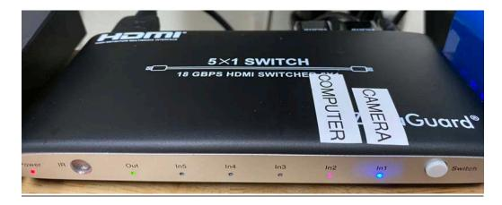
If you see your computer external monitor desktop on the teleprompter screen, you have the computer input selected. The In2 indicator on the HDMI switch marked as COMPUTER is blue:
