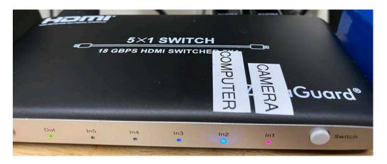
• You can switch between the inputs by **selecting the desired input In1 or In2 on the remote** or by pressing the **Switch** button until the desired input lights blue (you may need to circle through the inactive inputs).
